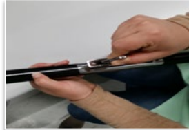
In most cases, you can re-align the latch by bending it by hand.
