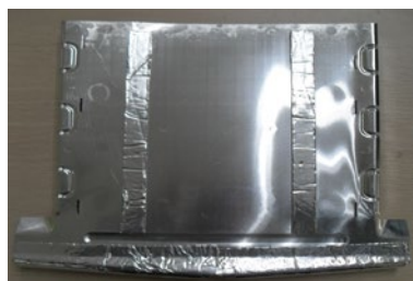
Foam strips installed (back and bottom)
