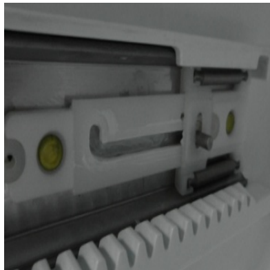
Pin in wrong position
