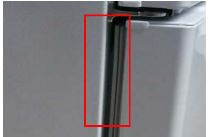
Gap between gasket and cabinet
