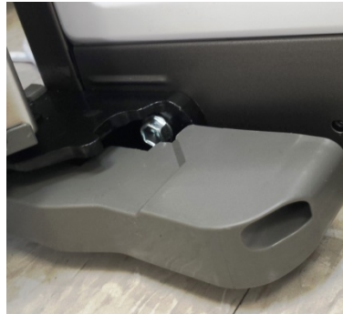
Hinge Cover Loose/Broken
