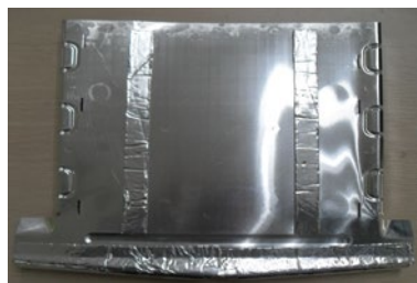
Foam strips installed (back and bottom)
