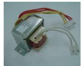
Low Voltage Transformer
