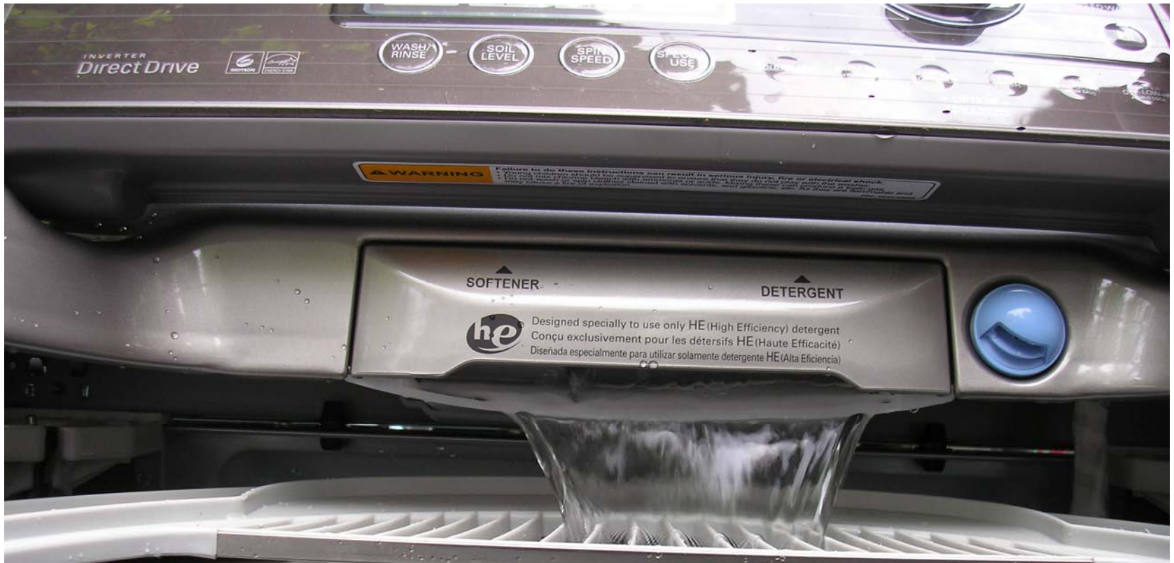
Main Water Inlet (Detergent & Softener)
